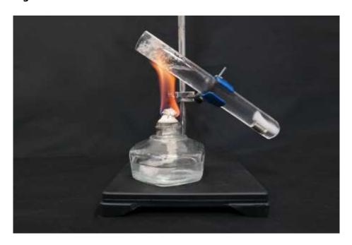
If you place ice at the bottom of a test tube and fix it so it doesn't float, and then heat the top part of the test tube, convection does not occur, and heat transfer is inefficient. In this case, heat moves only by conduction. Since water is a poor conductor of heat, the water at the top boils while the ice at the bottom remains unchanged.
